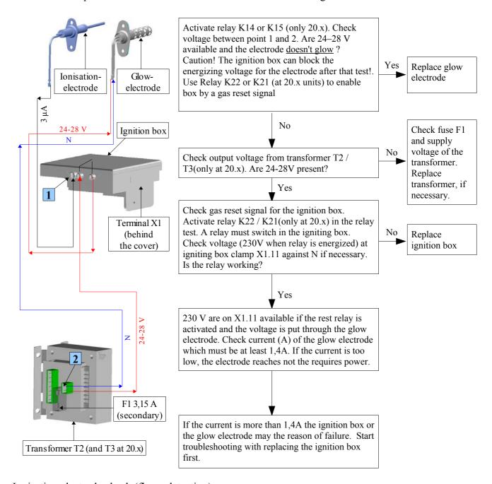
Ionisation electrode check (flame detection)
