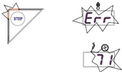
If the flame was not detected within 6 seconds after the gas valve was opened the procedure is stopped and the error **Err 71** is displayed. Please check that an external gas valve is opened. If a unit is started for the first time this error occurs several times until the air in the gas pipe is flushed out.
