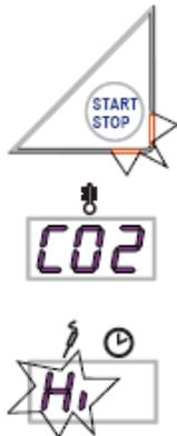
The CO2 has first to be measured at high power. After selecting **H1, H11, H12** press the START/STOP button.
