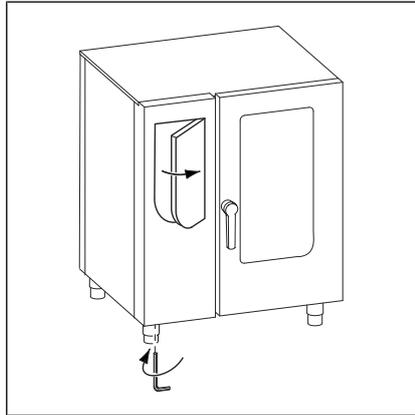
**Closing the control panel** Close the control panel by repeatedly pressing the left side (particularly in the upper left). The control panel locks noticeably at multiple points.
