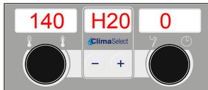
**Starting water test** → Press the "START STOP" button.
