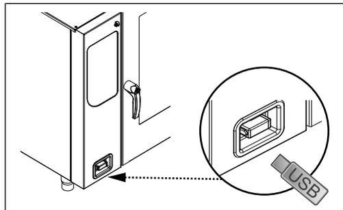
The USB interface is behind the cover on the bottom left of the housing.
