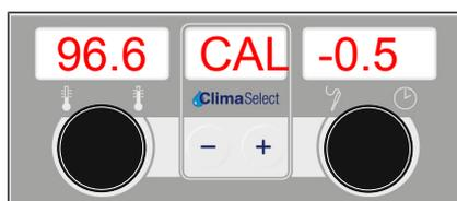
**Calibration** → Adjusting offset value with a rotary knob on the right.
