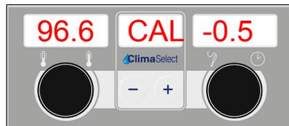
**Checking the calibration** → Press the "START STOP" button.
