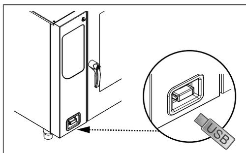
The USB port is located behind the cover in the lower left area of the housing.
