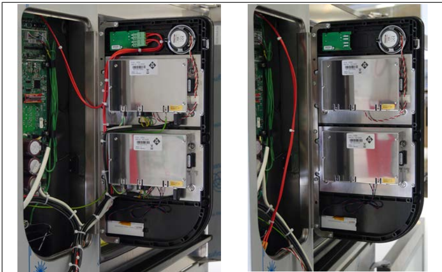
Image: Operating panel with and without cables
