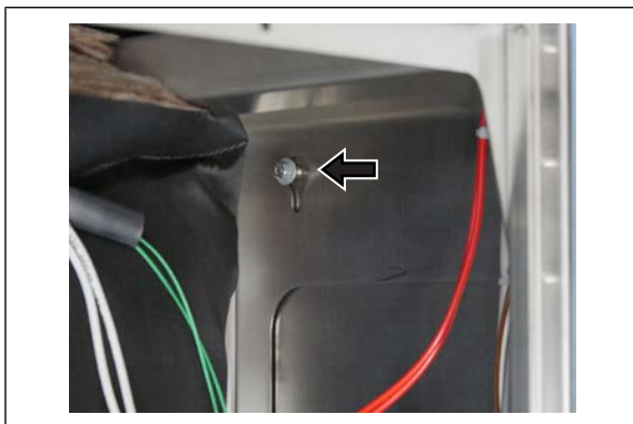
Image: Correct positioning of the pins
