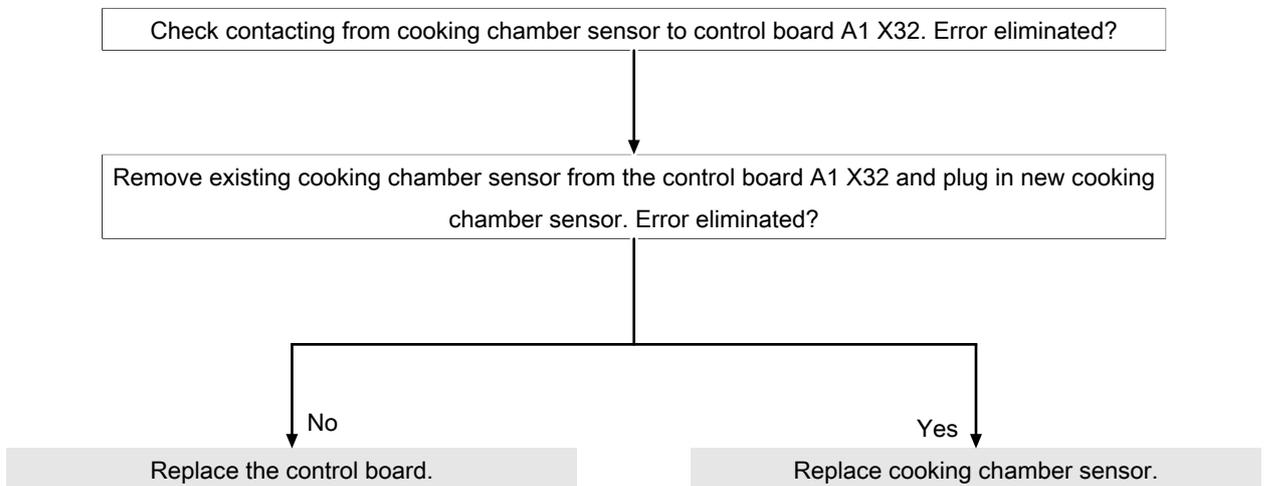
Alternatively, disconnect top cooking chamber sensor from A1 X31 for test purposes and connect to A1 X32 to see if the error "migrates".
