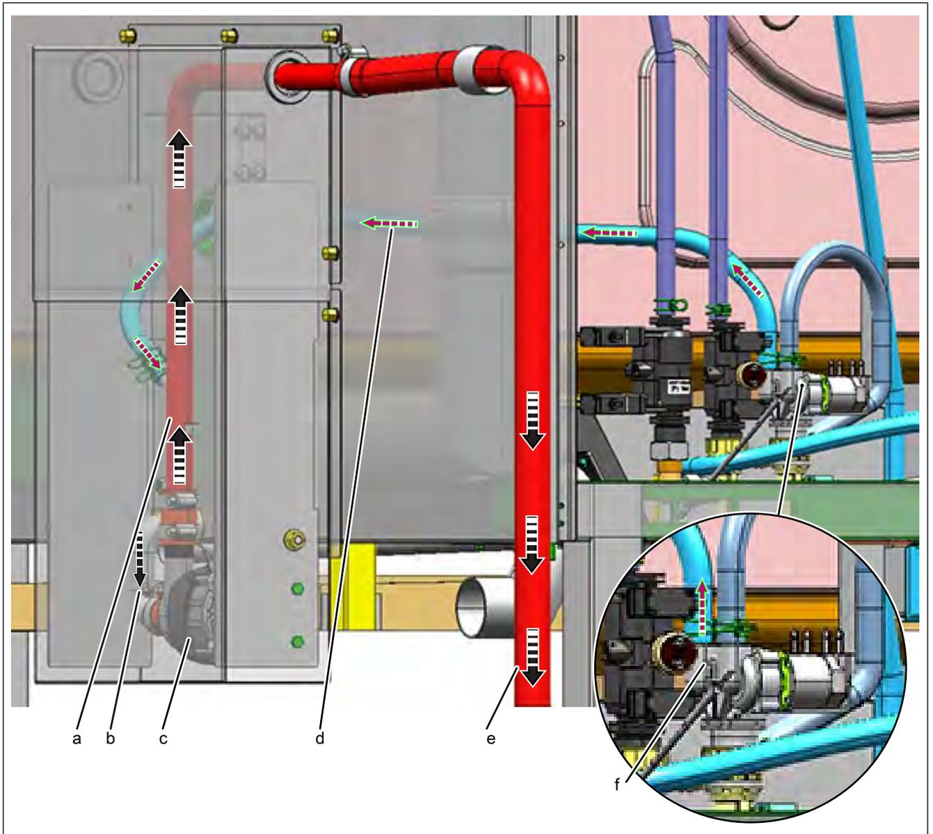
Image: Overview of grease drain system
