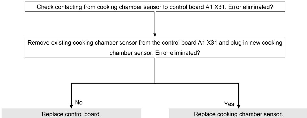
**Lower cooking chamber sensor faulty (697, 729)**
