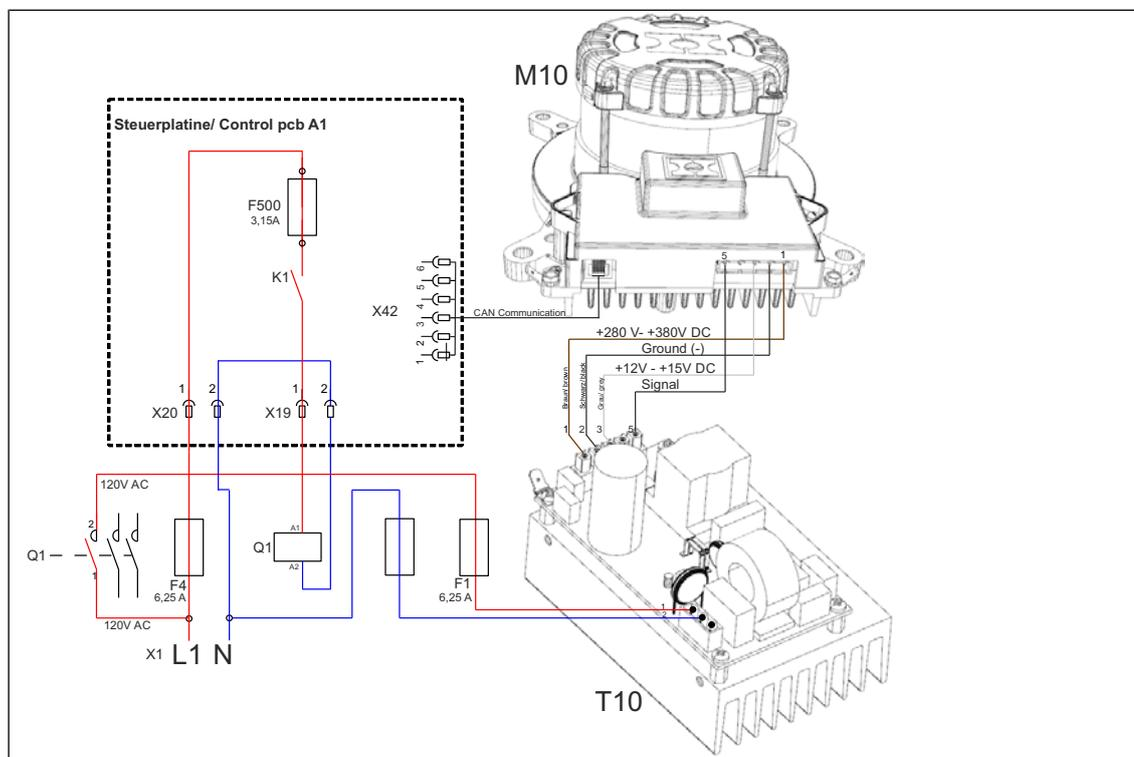
Image: Motor system 615,620,115, 120 Tabletop unit
