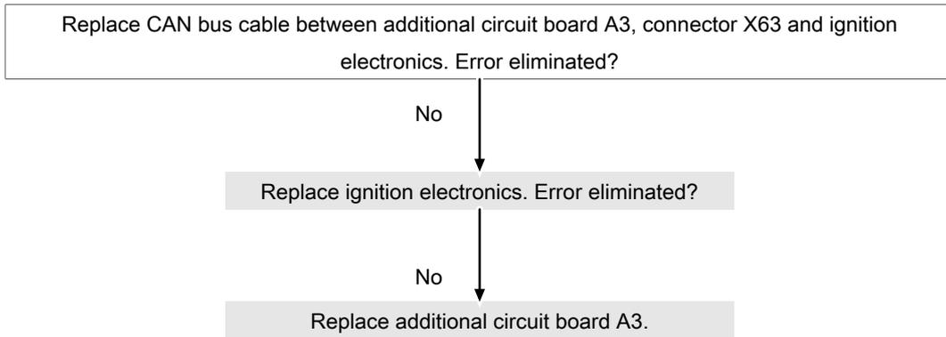
**Communication fault ignition electronics (top)(OTH\_ID26)**
