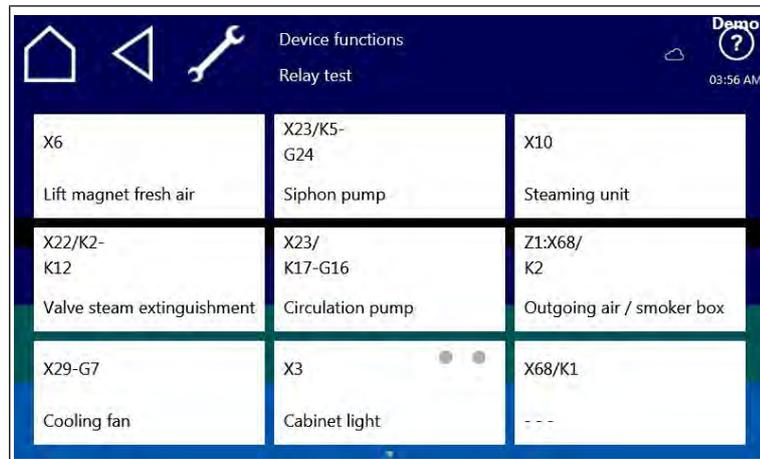
The cooking chamber door must be closed to control the G16 circulation pump.
