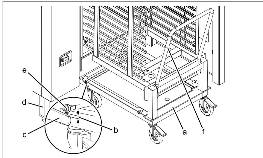
Image: Aligning tray trolley with insertion system
