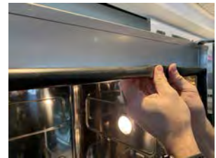
Image: Always press in the seal from the center outwards
