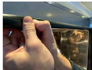
Image: Always press in the seal from the center outwards
