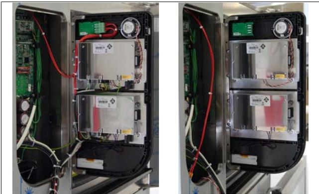
Image: Operating panel with and without cables
