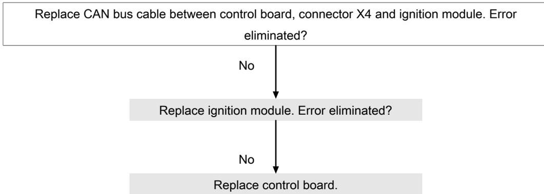
**Communication fault between I/O and ignition module (top)(OTH\_ID26)**
