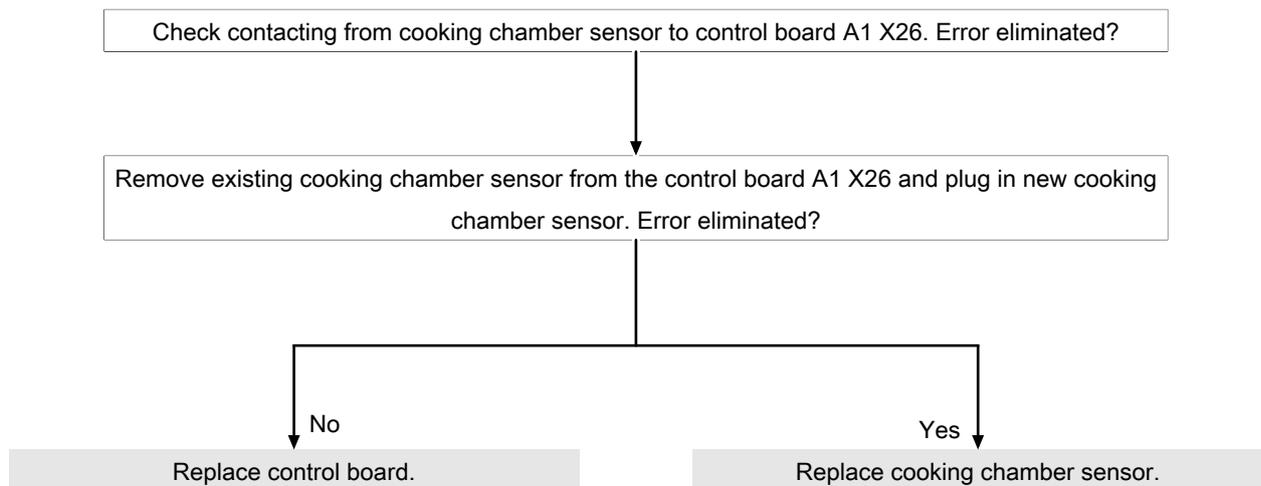
Alternatively, disconnect top cooking chamber sensor from A1 X25 for test purposes and connect to A1 X26 to see if the error "migrates".
