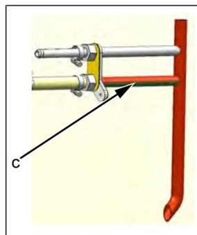
c Water supply pipe in the cooking chamber
