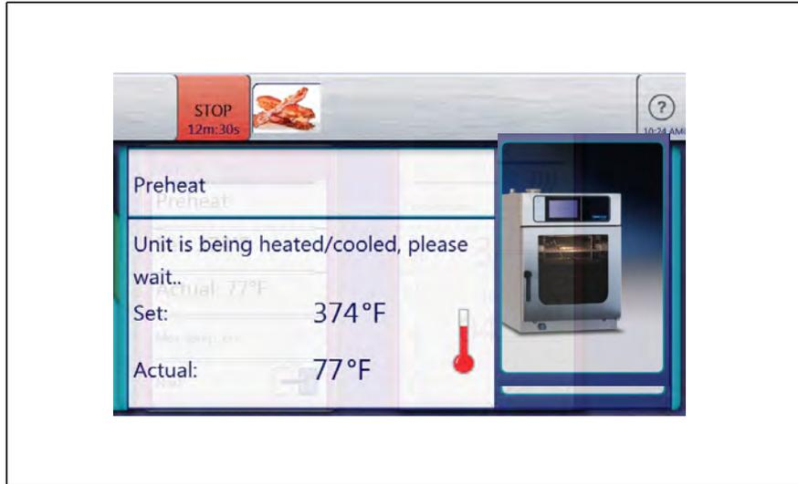
⇒ When the temperature has been reached, an audible alarm will initiate and the screen will show you that the temperature has been reached.
