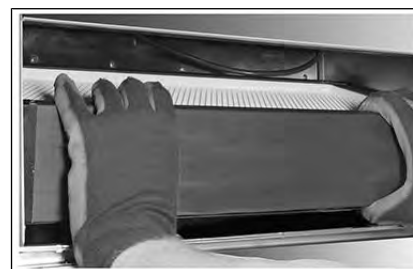
Image: Pay attention to the installation position of the air filter
