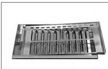
Image: Removing lower part of the filter holder and condensation baffles from the filter frame
