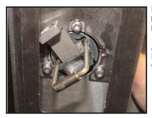
Place the handle onto the door and install the bottom two screws first and the top screw last.
