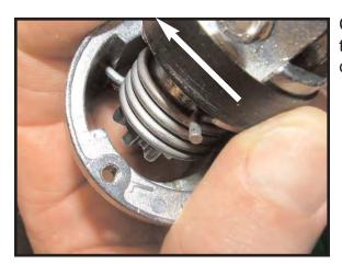
Carefully rotate the assembly clockwise until the other "pin of the sping lines up with the other notch in the housing.
