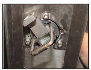
Notice that there are three screws. Remove the three screws using a T-15 torx driver.
