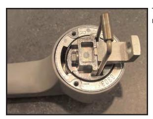
The door handle and mechanism can now be removed from the door.
