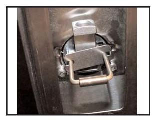
Install the metal spacer
