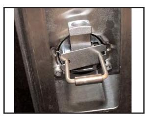
Now carefully remove the metal spacer
