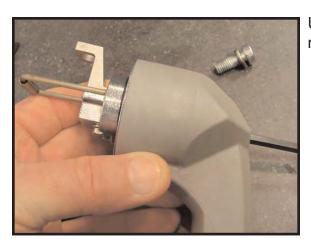
Using the Allen wrench, push out the mechanism.
