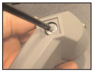
Remove the 5mm Allen screw
