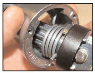
Insert the assembly into the housing. Be sure that the spring lines up with the notch in the housing
